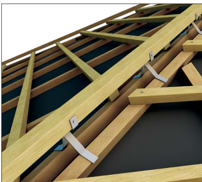
Option 1: Hip batten - installation with bracket
