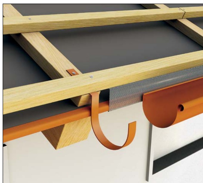
Option 1: Protection flashing going behind the gutter
