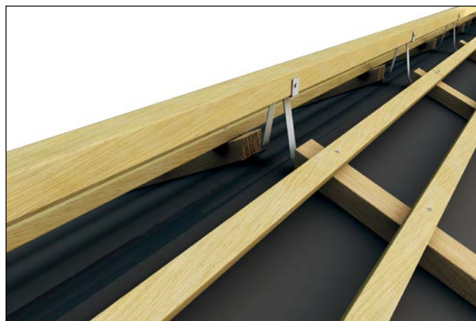
Option 1: Ridge batten - installation with bracket
