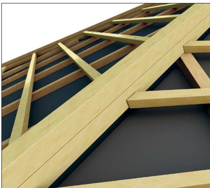
Option 2: Hip batten - installation with batten understructure
